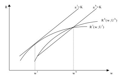
Separating equilibrium. The wage for high-type workers is determined at the intersection between the indifference curve for low-type workers and the iso-profit curve for firms attracting high-type workers.
